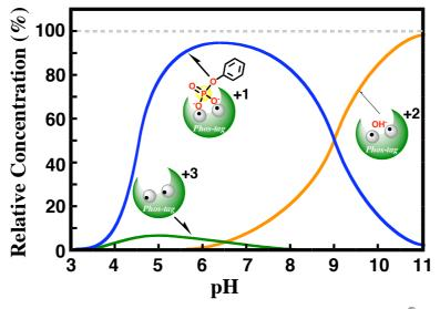
Species distribution for an aqueous solution of 10  $\mu$ M Phos-tag<sup>®</sup> 101 and 10  $\mu$ M phenyl phosphate at 25 °C with I = 0.10 (NaNO<sub>3</sub>).
