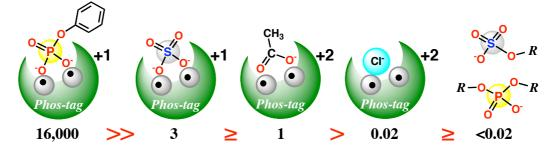
Phos-tag<sup>®</sup> 101 series (+3 ion) selectively captures a phosphomonoester dianion (-2 ion). The electric charge of the Phos-tag<sup>®</sup> 101–phosphomonoester<sup>2–</sup> complex is +1, which is suitable for MALDI-TOF Mass analysis. Binding of borate, nitrate, and perchlorate is negligible in H<sub>2</sub>O at room temperature.
